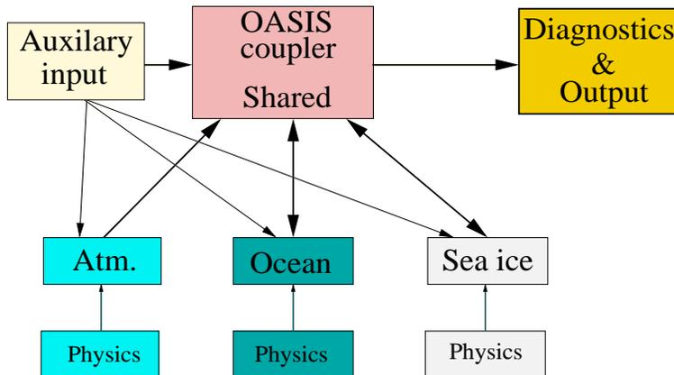
Figure 2: Sequence of numerical coupler for a three component ocean-ice model with data atmosphere.
