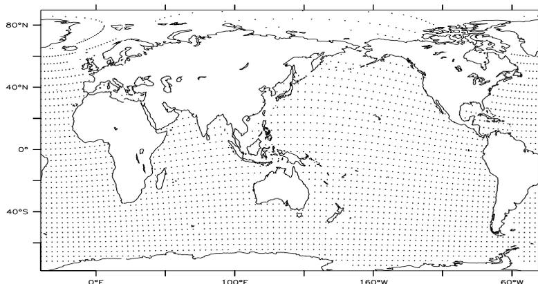
Figure 6: Displaced pole grid used for the ocean and sea-ice sub-models. Latitude and longitude lines are only shown every  $1^\circ$ .
