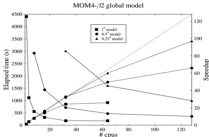
Figure 4: Parallelisation efficiency of MOM 4 $\beta$  on the APAC AlphaServer SC facility with two dimensional domain decomposition.
