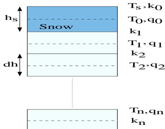
Figure 1: Vertical conduction of thermal energy through the sea ice and snow.
