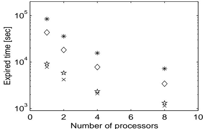
Figure 5: Execution time for the sea-ice sub-model and selected components when running on an SGI3400 with 1, 2, 4, and 8 processors. (See text for details.)
