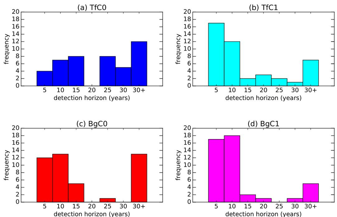
**Figure 2.** Distributions of the estimated time horizon over which the SAI influence would become detectable in the temporal pattern of global-mean SATs after 2020 by using the (a) TfC0, (b) TfC1, (c) BgC0 and (d) BgC1, respectively, at the 10% level. The results are more sensitive to the choice of filter than to the detection methods alone.
