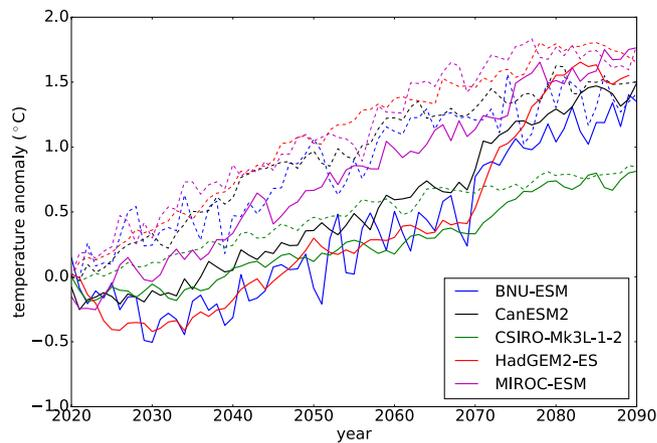
**Figure 3.** Ensemble-mean annual-mean global-mean SAT anomaly (relative to the corresponding 2020 levels) time series in G4 (thick solid line) and RCP4.5 (dashed line) from BNU-ESM, CanESM2, CSIRO-Mk3L-1-2, HadGEM2-ES and MIROC-ESM, respectively.
